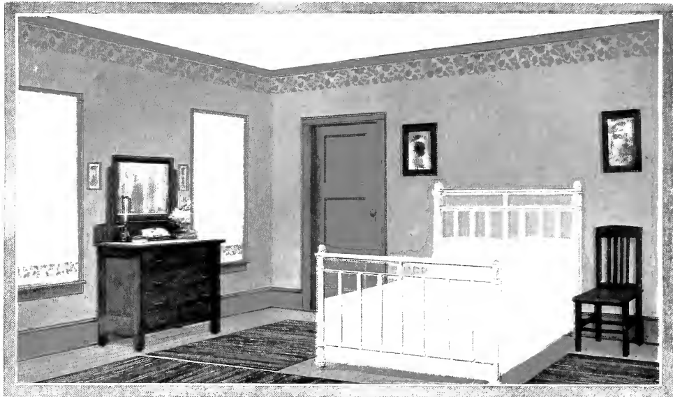
Specification— Ceiling , S-W Flat-tone, Cream. Wall , S-W Flat-tone, Old Gold. Stencil , No. 10. Woodwork , Natural Pine; finished with S-W Excello Varnish. Floor , Natural; finished with three coats S-W Mar-not Varnish.
